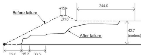
Figure 2. Failure of Barahona tailings dam, (Agüero, 1929).
