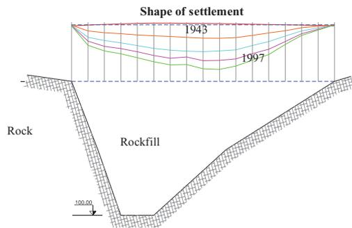
Figure 33. Vertical settlements along the crest of Cogoti Dam.
