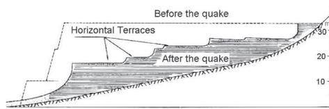
Figure 3. Failure of El Cobre tailings dam, (Dobry et al., 1967).
