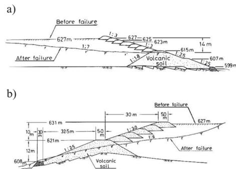
Figure 4. Failure of Mochikoshi tailings dams. (a) Dike N° 1 and (b) Dike N° 2, (Ishihara, 1984).
