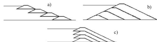
Figure 1. a) Upstream, b) downstream and c) center-line methods of construction.
